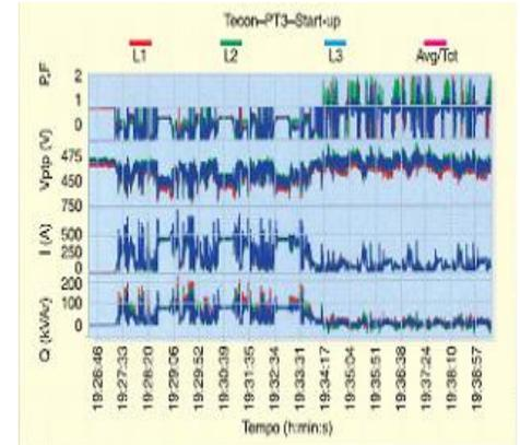
Measurement on Crane Startup
