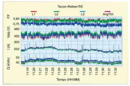
Figure 3 Duty Load Cycle
